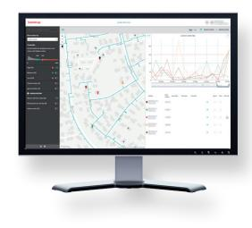
Leaks can be caused by a variety of reasons and often difficult to detect. With acoustic noise data from your water meters, leaks can now be detected in an entirely new way. Leak Detector, the analytics module in conjunction with the flowIQ® 2200, enables you to locate leaks based on acoustic noise levels registered by the meter, which means time can be spent fixing leaks instead of searching blindly for them.
