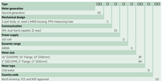
Fibre gaskets are supplied along with flowIQ® 2-part body meters. The features included in the Type Number cannot be changed once the meter has been produced.
